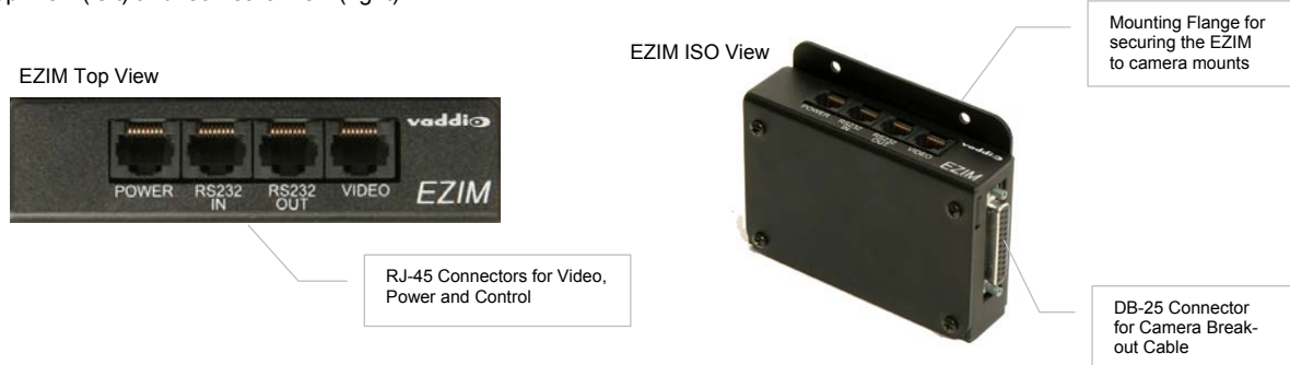
Figure 3: EZCamera Interface Module (EZIM) with four (4) RJ-45 connectors for POWER, RS-232 IN & OUT and VIDEO (SD with IR), Top View (left) and Isometric View (right)
